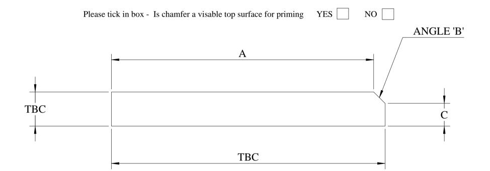
CUSTOMER TO CONFIRM DIMENSIONS A+B+C INCLUDING PRODUCT WIDTH AND THICKNESS. WHEN DIMENSION C=0, ANGLED CUTTER MUST BE SET ON SIDE HEAD!
